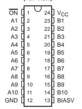
The SN74CBTS6800 is organized as one 10-bit switch with a single enable  $(\overline{ON})$  input. When  $\overline{ON}$  is low, the switch is on, and port A is connected to port B. When  $\overline{ON}$  is high, the switch between port A and port B is open. When  $\overline{ON}$  is high or  $V_{CC}$  is 0 V, B port is precharged to BIASV through the equivalent of a 10-k $\Omega$  resistor.
